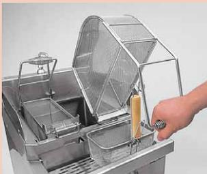
It reduces the burden of worker when turning the boiling baskets over.
