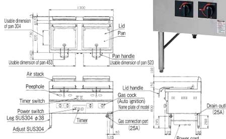
● SUS304 is used for pipe legs and adjust.
